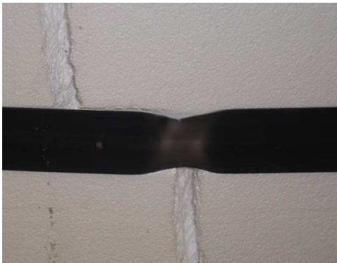
Figure 20. Furring Assembly Failure, "Necking" (left) and Fracture (right)
