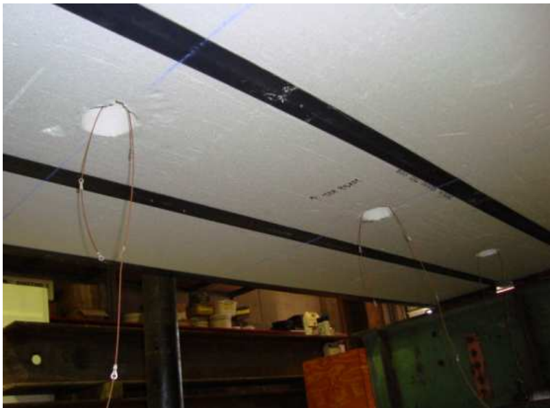
Figure 15. Displacement Transducer Attached to the Specimen
