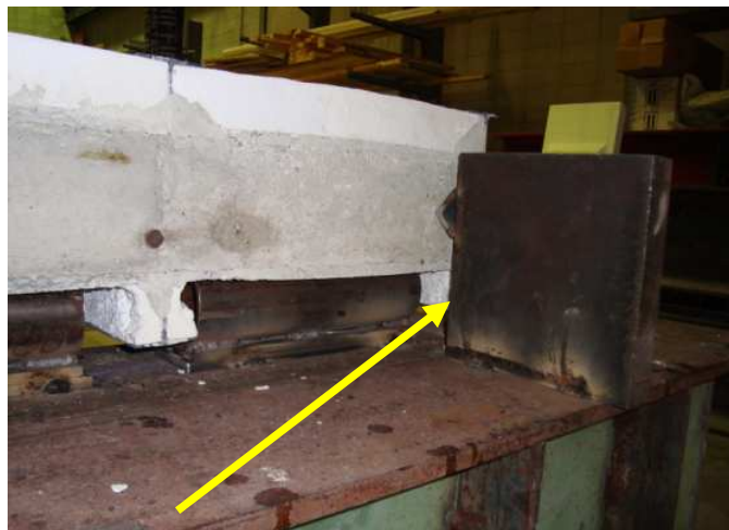
Figure 16. Fabricated Abutment on Pinned-End
