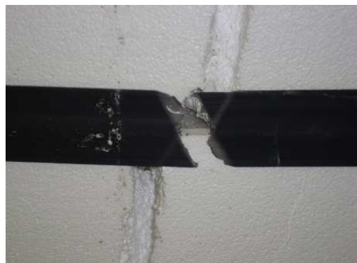
Figure 20. Furring Assembly Failure, "Necking" (left) and Fracture (right)
